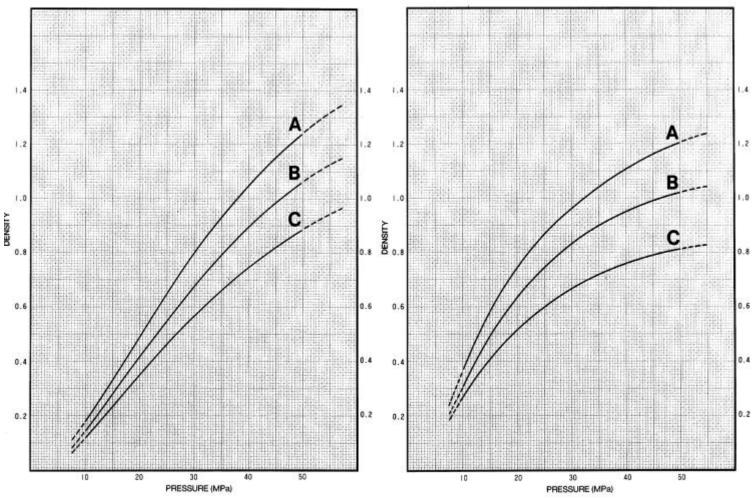
As the pressure ranges indicated by the broken lines in the above graphs may exceed the permissible error range, they should be used for reference only.
