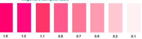
Even if Prescale can offer a "visual" direct imaging of pressure distribution and magnitudo, better results are achievable by mean of shown standard charts and magenta's colour table. In choosing the proper curve (\*), check for ambient temperature and humidity conditions and make sure which area is the closest to your experiment (see side chart). For example, if the room temperature is 25°C and the humidity factor is 60% RH, acquire the pressure using the B curve in standard chart.
