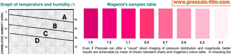
results are achievable by mean of shown standard charts and magenta's colour table. In choosing the proper curve (\*), check for ambient temperature and humidity conditions and make sure which area is the closest to your experiment (see side chart). For example, if the room temperature is 25°C and the humidity factor is 60% RH, acquire the pressure using the B curve in standard charts.
