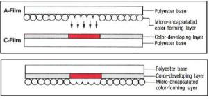
with distribution and "density" of magenta colour depending by true pressure distribution and magnitude. When microcapsules are broken, their material is released and it react with the colour developing material and this process will cause magenta colour forming. Through PSC technology (Particle Size Control), microcapsules are designed to react to various degrees of pressures, releasing their colour forming material at a density that correspond to specific levels of applied pressure.
